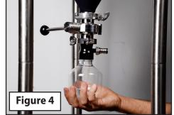
Slowly loosen the collection bottle to allow air pressure to release out the top.
