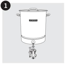
**Step 1** Begin by installing valve assembly so that the handle points away from the system when the valve is open. Tip: In order to turn the valve handle, you must first pull up on the handle lock.
