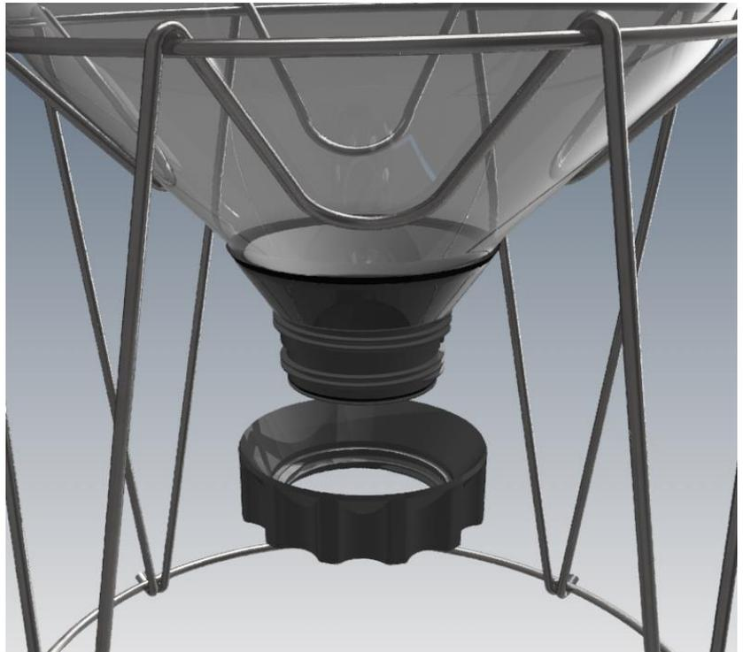
3. Locate the butterfly dump valve and screw this onto the spigot. This is a **RIGHT HAND THREAD**. Screw this onto the spigot firmly. Once again do not over tighten this fitting as additional tightness will not improve the sealing performance.
