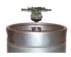
1. Align lug locks on coupler with lug housing in top of keg; insert coupler.
