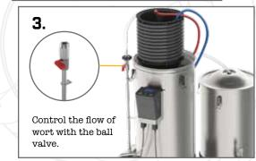
Turn the cooling water on. Once connection D runs cold, switch the pump off and place it inside the clean and sanitised fermenter. Always try to keep the fermenter sealed. Add yeast as instructed on recipe. Take an OG reading of cold wort.
