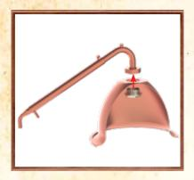
1. Attach the copper condenser arm to the copper dome by removing the nut and 0 ring from the base of the condenser. Sit the condenser on the dome and screw the nut and 0 ring back into the condenser (check the lid isn't spinning anymore) to firmly attach the dome to the condenser.
