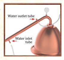
3. Attach the tubing for the water cooling of the condenser. The thin tube is for the outlet water and connects near the top of the condenser arm and takes the water back to the sink. The thicker tube connects to the water inlet near the tip of the condenser arm, with the other end connecting to the tap.
