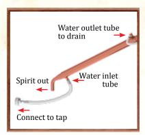
4. Briefly turn on the cooling water supply to ensure there are no leaks in the system. Check again that the water goes in at the end where the spirit comes out and that the water comes out closest to the top of the lyne arm (at the end near the thermometer probe).
