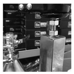
Please be sure to put a washer between The bottom of the leg / threaded insert and the nut. Install your caster as shown in the figure above. It is important to have the washer as shown in order to distribute force evenly across the leg bottom and around the threaded insert.
