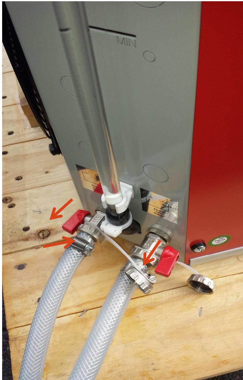
Pic. 10: Reconnect the tube/hose to the chillers outlet. Then open both valves (The valves are open when they are parallel to the tube, see arrows).
