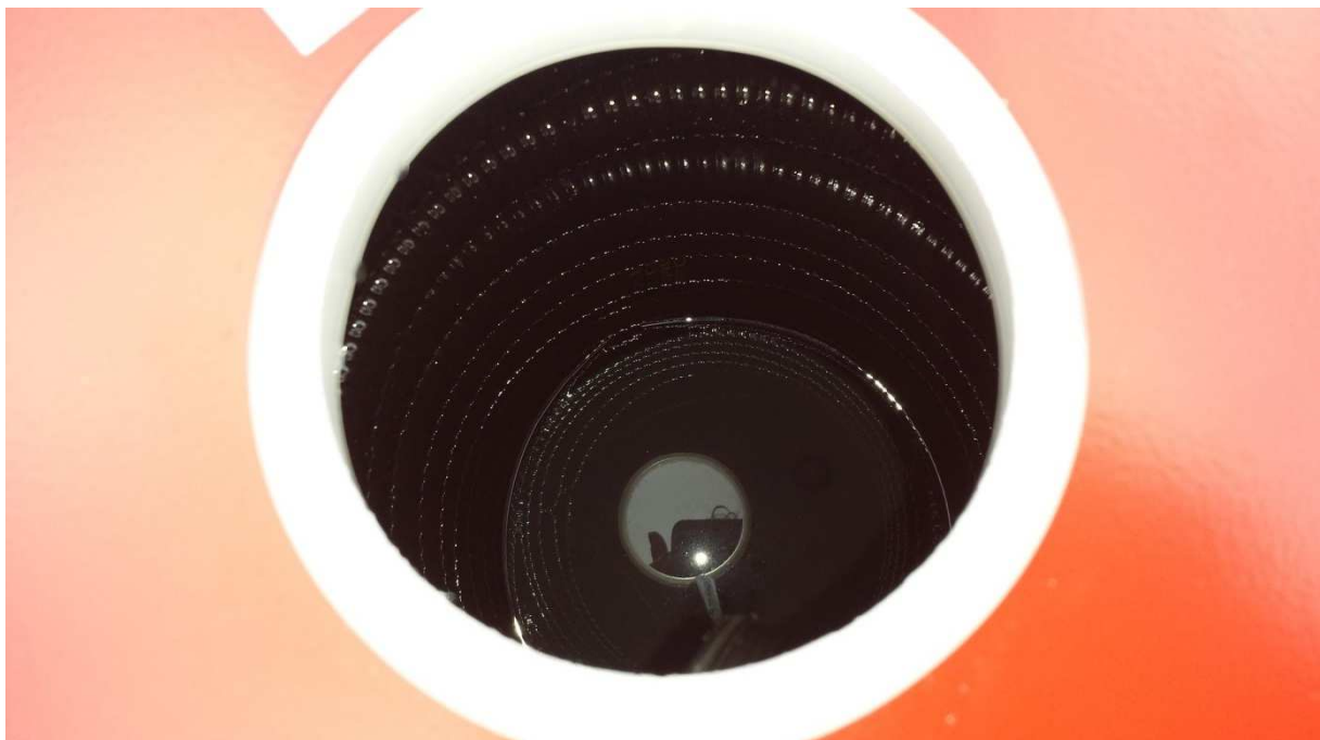
Pic. 3: View inside of the open tank – the heat-exchanger (evaporator) in spiral type is visible
