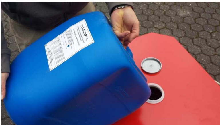
Pic. 5: Add 'food-safe' grade glycol (anti-frost protection) to the water. The concentration of the Glycol in the total quantity of water in your system depends on the water temperatures you want to set your Chilly to produce, and the instructions from the Glycol manufacturer. Typically, you need to have about 25% - 30% of Glycol part in the total quantity of water in your system. (Necessary for low temp Chillys, if ambient temperature can reach negative temperature or in case of cooling below +8°C is needed)
