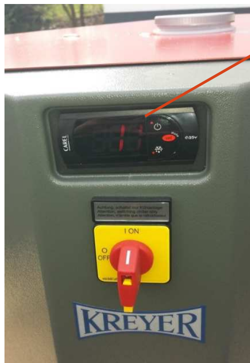
Pic.15 (left): Adjusting the Set-Temperature ( this picture is in Celsius degrees, in the next page and in the official manual you will find how to change your unit to show F° Fahrenheit degrees)
