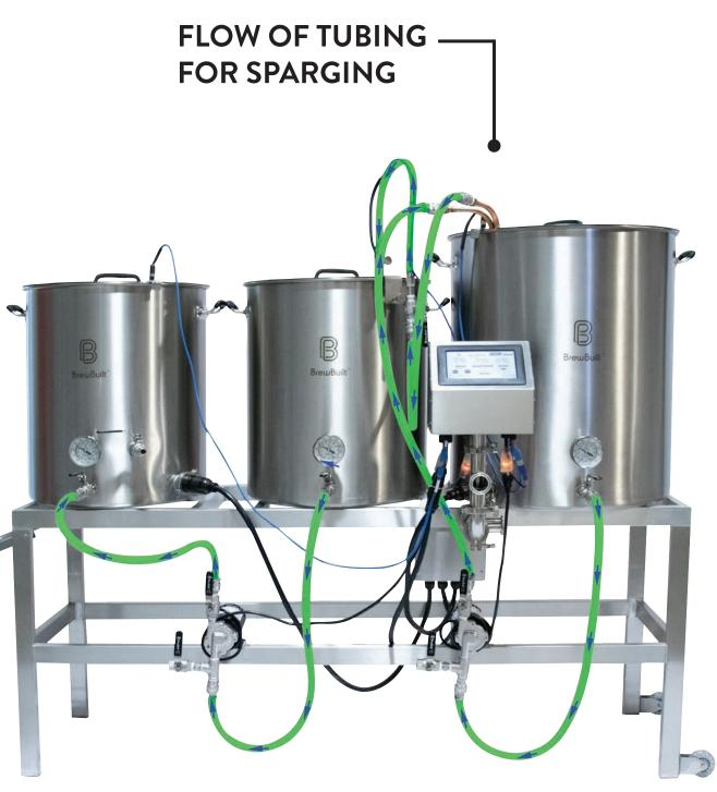
If you set the power slider on the Sparge Screen to 50% it will keep your HLT warm while preheating the boil. It will not turn on the boil element till the float switch reads UP and it will kill the HLT element when the HLT float reads DN.
