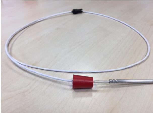
Afterwards, the sensor cable is inserted through the rubber plug (slightly dampen sensor and plug, so that it can be pushed through easier) and then the rubber plug is inserted very powerfully in a rotating motion so that the cable entry is firm and sealed. If necessary, pull the plug from the reverse side.
