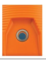
**Step Three** — Using a black felt tip pen (2), trace inside the stainless washer (4c), creating a template for filing out the hole. When you are done tracing you will have what looks like a crescent moon shape (see far right image).
