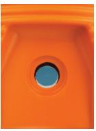
**Step Four** — Using a general purpose half-round file (1), begin to slowly expand the traced spigot hole. **NOTE**: Be careful to not file out too much, as going outside of the template will result in a non-sealing spigot!
