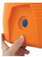
Step Five — Once the hole is filed out and cleaned of debris, push your bulkhead (4a) through the newly expanded spigot hole on the outside of the cooler. On the inside of the cooler, replace the red gasket (4b), then the stainless washer (4c), and finally, thread the lock nut (4d) onto the bulkhead, sealing the system.
