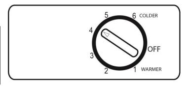
Caution: If you powered off the unit, please wait at least 5 minutes before powering it back on. This kegerator has one control knob located on the left of the inside of the cabinet. Turning the knob to the right or left will make the unit colder or warmer respectively; 1 being the warmest and 6 the coldest.
